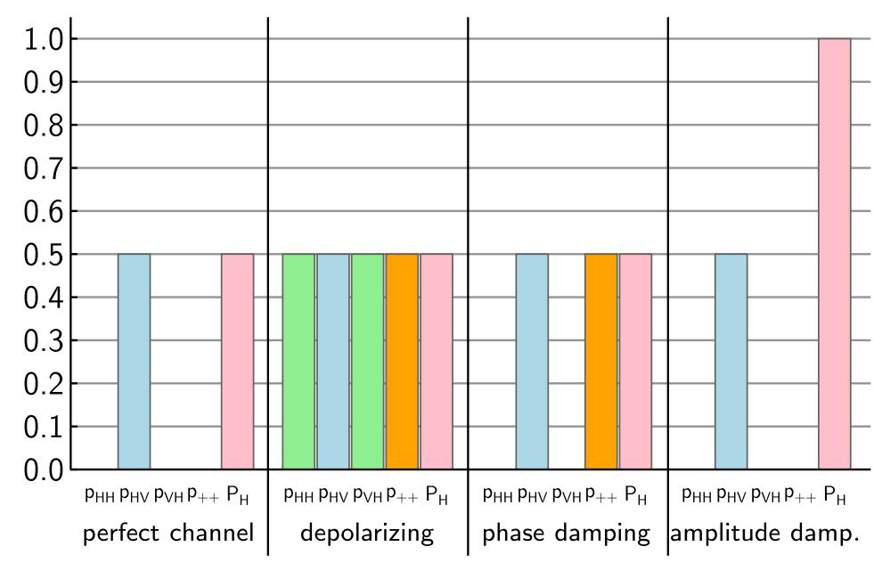
Channel errors were simulated by randomly applying polarization transformations together with the required local projections. Each error deviates the collectibility from its theoretical minimum. By observing individual outcomes of respective measurement settings, one can identify the type of occurring error (each channel has a characteristic fingerprint).
