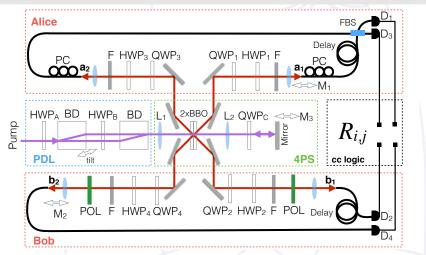
constructed a quantum relay using linear optics
