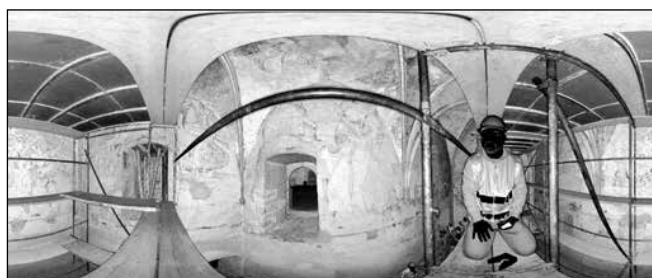
Fig. 3 Preview mode, allowing to choose the horizontal and vertical angle of view for subsequent full-resolution scans
